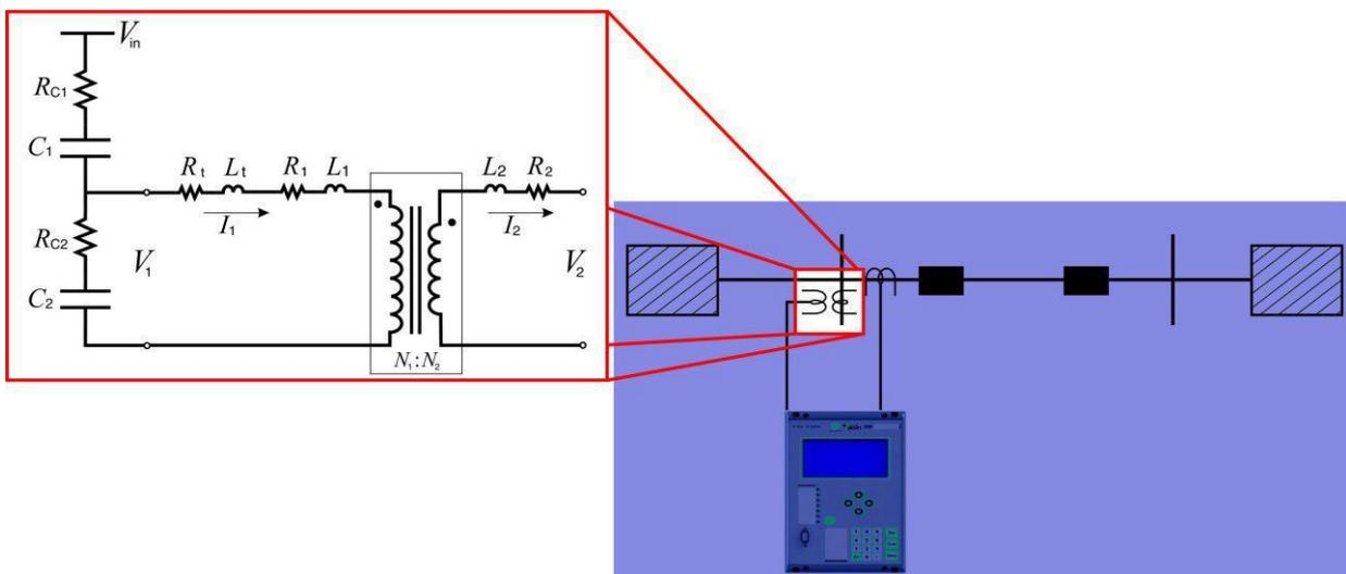
Figure 1: equivalent circuit of the CVT.
