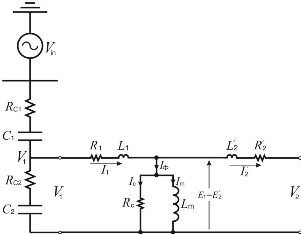
Figure 5: CVT equivalent circuit with transferred electrical quantities (Sen 2007).
