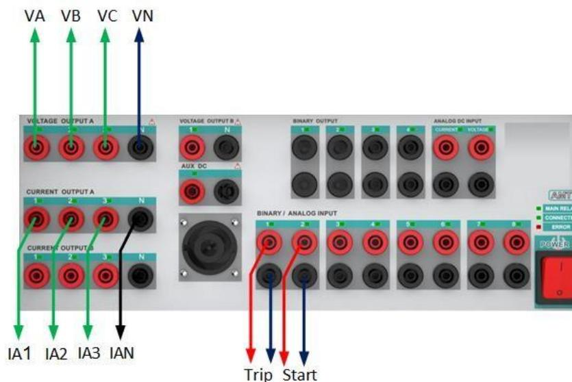
**Figure 7:** Connections to the VTFF monitoring unit testing.
