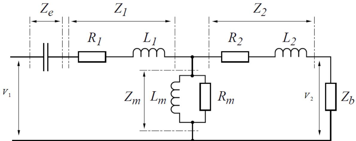
Figure 6: Simplified CVT equivalent circuit (Sjövall 2005).
