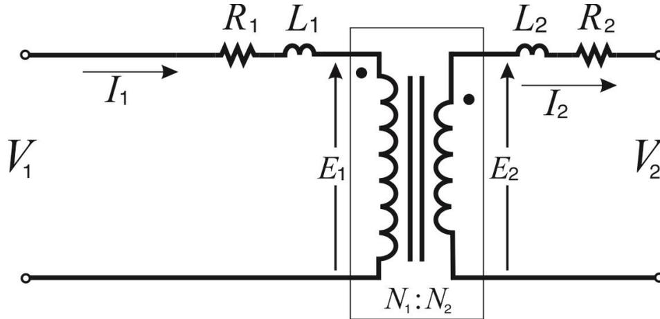
**Figure 3:** The equivalent circuit of a single-phase transformer (Sen 2007).
