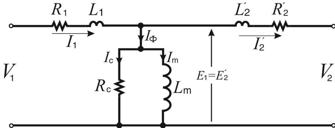
**Figure 4:** The equivalent circuit of a single-phase transformer with electric quantities transferred to the primary side (Sen 2007).
