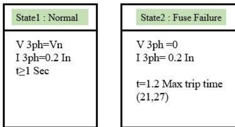
**Figure 9:** States related to the voltage unreliability test for all three phases.
