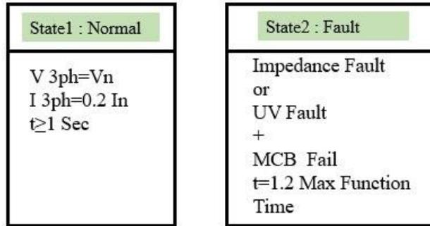
Figure 10: States related to Blocking the protective function with MCB Fail Auxiliary contact
