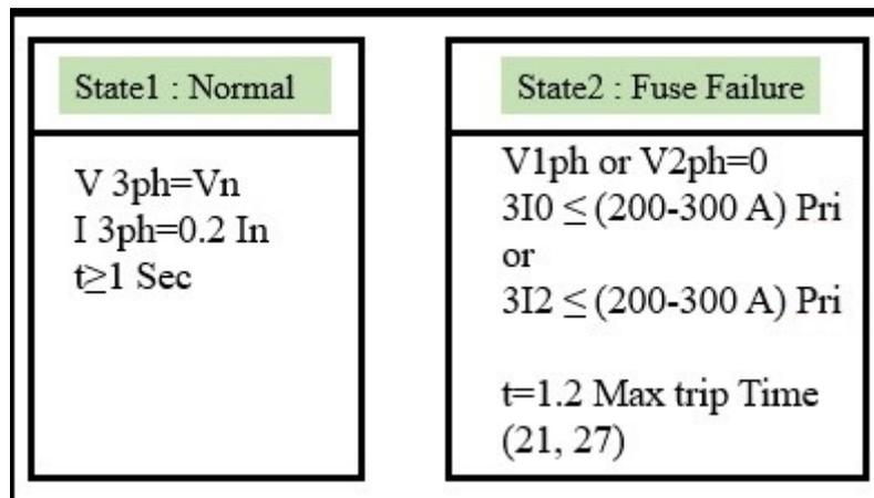
**Figure 8:** States of unreliabing one or two phase voltage Testing.
