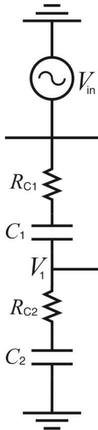
**Figure 2:** equivalent circuit of CVD.
